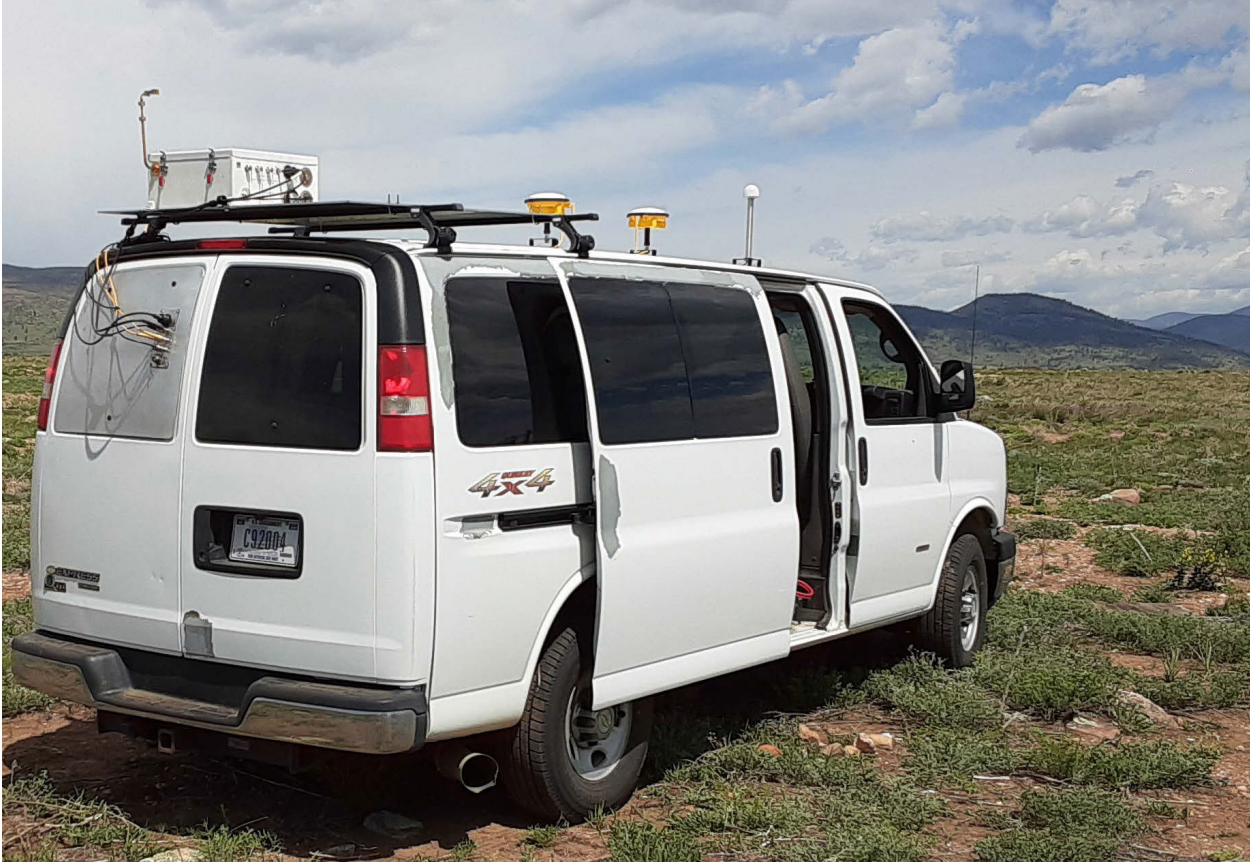
Figure 5. Measurement system vehicle: ITS modified Chevrolet Express 3500 passenger van. Credit: ITS Staff
