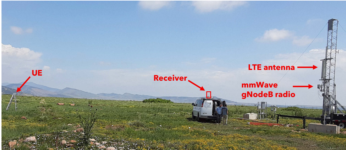
Figure 7. Location of the mmWave gNodeB radio mounted on the tower, measurement system vehicle, and UE. Credit: ITS Staff.
